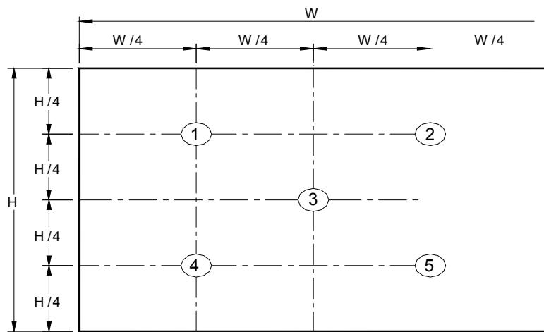
Note 3: The luminance uniformity of 5 points is defined by dividing the minimum luminance values by the maximum test point luminance
