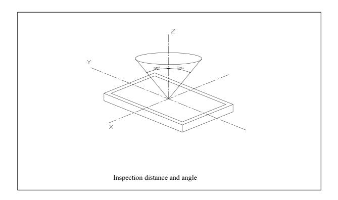
Inspection should be performed within angle $\varphi(\varphi)$  is usually 30°) from Z axis to each X and Y. Inspection distance in any direction within  $\varphi$ must be kept 30±5cm from the display surface.
